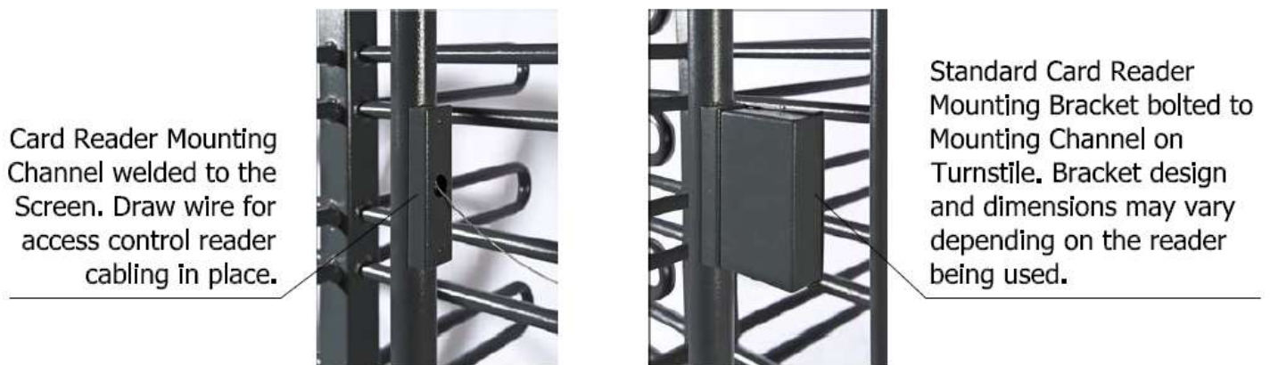
Figure 7: Card reader mounting channel, draw wire and reader bracket
